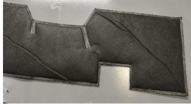
Insulation Pad At Engine Area
